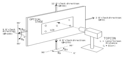
Figure 3. Response Time Testing
