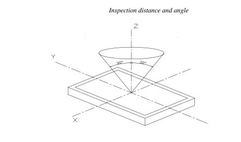
Inspection should be performed within angle  $\phi(\phi)$  is usually 30°) from Z axis to each X and Y. Inspection distance in any direction within  $\phi$  must be kept 30±5cm from the display surface.
