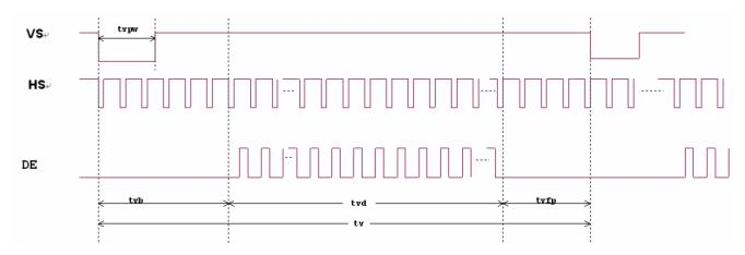
Vertical input timing diagram
