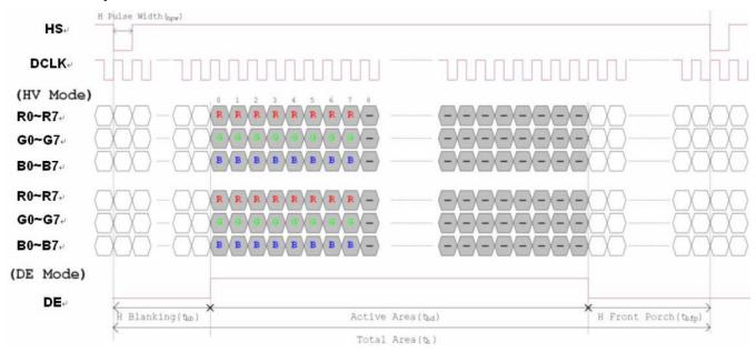
Horizontal input timing diagram
